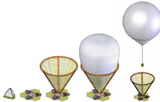
Shielded Mars Balloon Launcher (SMBL) deployment sequence
