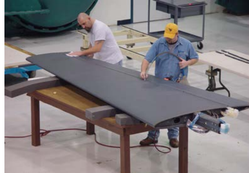
Technicians at Aurora Flight Sciences' West Virginia plant put the finishing touches on the Global Hawk V-tail.
