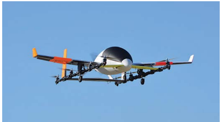
Subscale vehicle demonstrator of Aurora's eVTOL aircraft achieves successful test flight, incorporating transition from vertical take-off to forward cruise.
