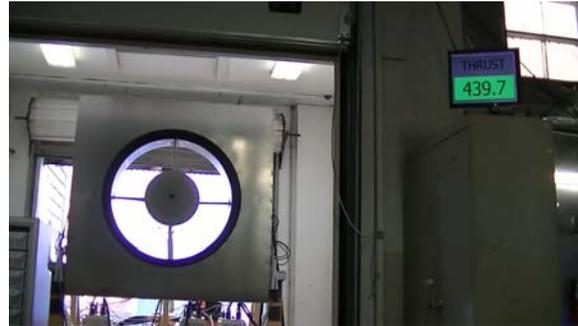
Aurora, ThinGap, and Trust Automation electric lift fan thrust test
