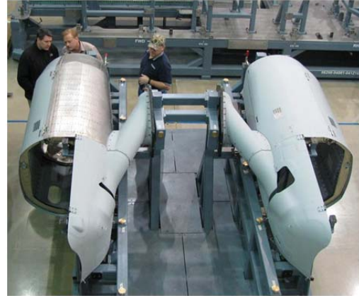
Nacelles deliverables installed on final assembly structure - pictured from left to right, Adam Naternicola, CH-53K DPM, Eugene Matthews, IPT Lead, and Robbie Robinson, Production Supervisor.
